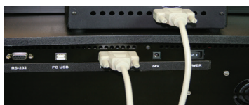
Figure 117. Cable connection of injector system to GloMax® Explorer Instrument.
