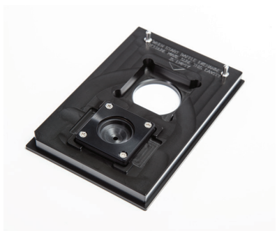
Figure 94. Aperture Plate with 384-well Aperture Fitting in the front position.
