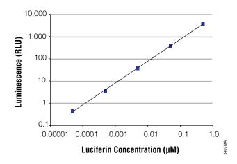
**Figure 3. The correlation between luminescent signal and p-luciferin concentration.** Luciferin was titrated in MAO Reaction Buffer and mixed with an equal volume of reconstituted Luciferin Detection Reagent. The luminescent signal was measured 20 minutes after reagent addition. For all samples n = 4, and the standard deviation is smaller than the data points shown.
