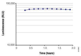
**Figure 9. The luminescent signal is stable in Step 2.** In a 50µl reaction, 40µM MAO Substrate was incubated with 2µg of protein from microsomes containing MAO-A for 45 minutes. After adding an equal volume of reconstituted Luciferin Detection Reagent, the luminescent signal was read repeatedly over 2 hours. Similar trends were noted in experiments with MAO-B.
